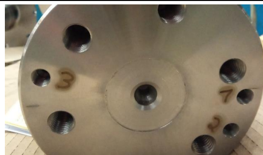
figure 9 output shaft: labelling with etching pen for three drilling holes
