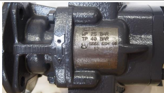
figure 17 pump (hard stamping)
