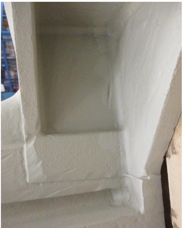
constriction at the transition, machining marks
