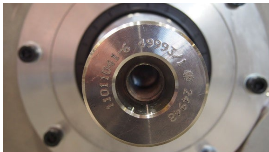
figure 7 drive shafts, output shafts without flange: on the outer end face intermediate shaft without flange: end face
