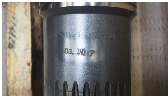
figure 13 pinion shaft: behind the run-out of the driving gearing
