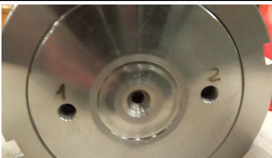
figure 8 output shaft: labelling with etching pen for two drilling holes
