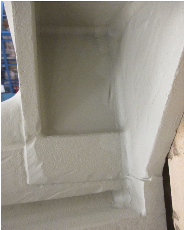
constriction at the transition, machining marks
