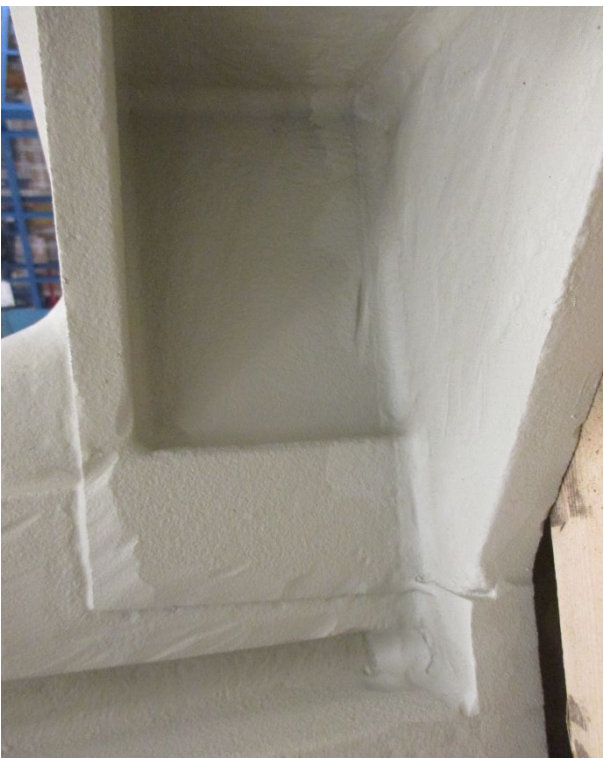
constriction at the transition, machining marks
